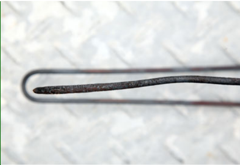
This is a burst core tube from a boiler matrix.
